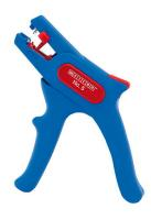
The WEICON Wire Stripper No. 5 has an adjustable length stop from 5 – 12 mm. This allows all flexible and solid conductors of 0.2 - 6.0 mm<sup>2</sup> (24 – 10 AWG) to be stripped. The length stop can be removed if required. An easy-to-access side cutter is integrated into the tool and can be used up to a cable diameter of 2 mm. It also has exchangeable blades.
